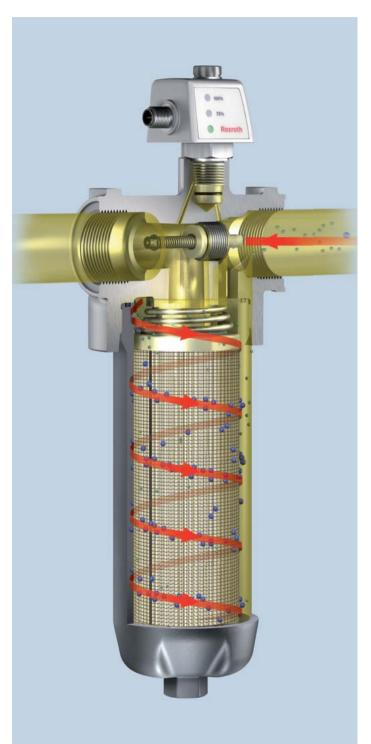
Filters guarantee high reliability in hydraulic machines and equipement. As part of a holistic filtration concept Rexroth has completely revised the filter material design. The focus of the development was to increase the dirt holding capacity compared to previous versions. This increases the changing intervals and reduces the maintenance, material and disposal costs.
